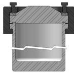
4660 Cross Section with Flat Gasket Seal
