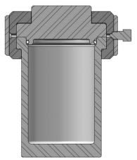
47600 Cross Section with O-ring Seal
