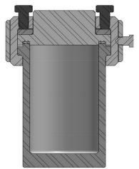
4760 Cross Section with Flat Gasket Seal
