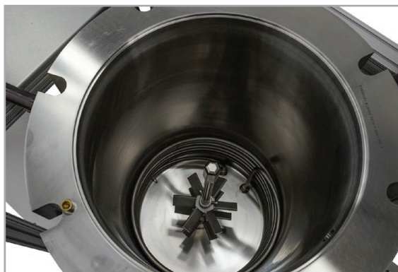
View of Stirrer and Spiral Cooling Coil
