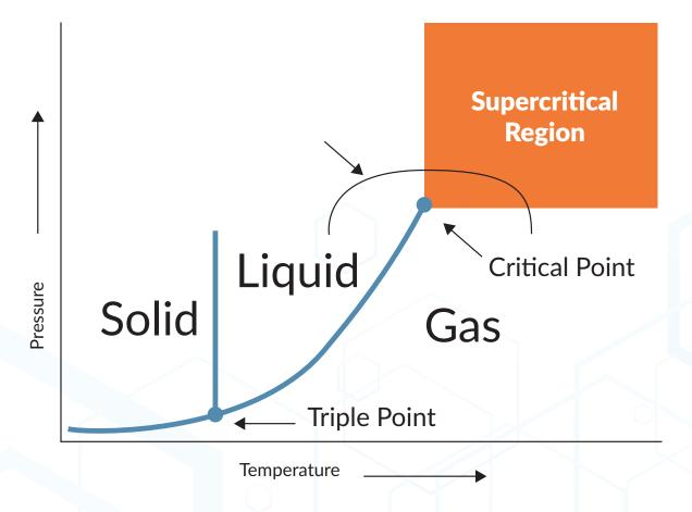
Figure 1–1: Supercritical CO2 is tuneable without changing phases
